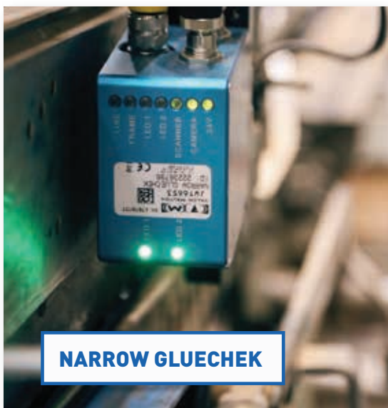
Double camera installation for back side inspection to detect glue residues
